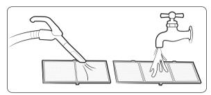
Clean the air filter with a vacuum cleaner or soft brush. If dust is too heavy, then rinse it with running water and dry it in a ventilated area.
